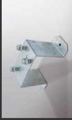
Spare wheel bracket (loose)
