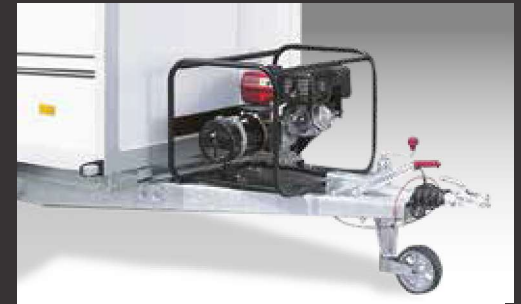
Power generator on the drawbar
