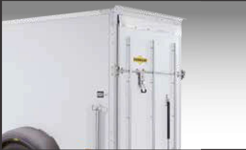
Ramp wall instead of rear door
