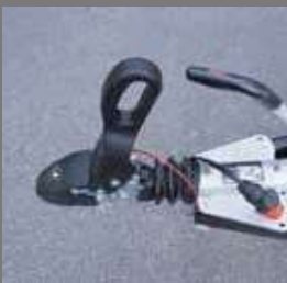
Safety coupling with track stabilisation
