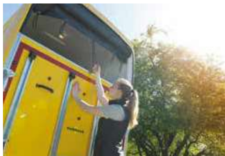
The tinted and five-way adjustable vent windows provide an optimum air supply. The exclusive Humbauro wind deflector offers draft-free ventilation and continuous air circulation.
