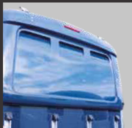
GRP wind flap with integrated third brake light (optional) for Baljos®, Xanthos®, Zephir® and Maximus®
