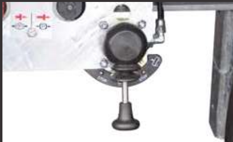
Air suspension with lift/lower function
