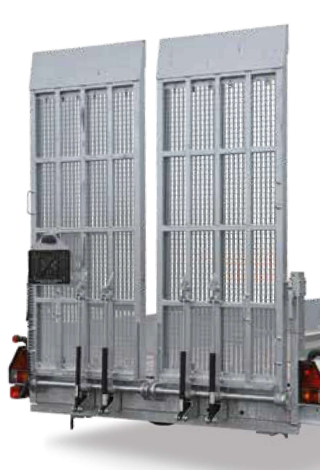
One-piece, wide ramps with steel grating
