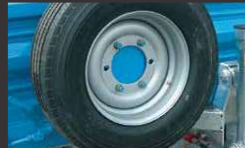
Spare wheel holder on the front wall (only in combination with steel front walls)
