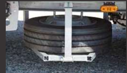
Spare wheel holder as basket under the cargo bed
