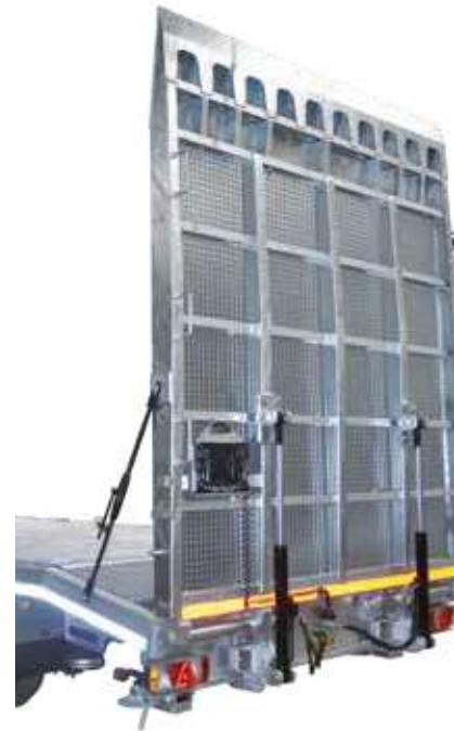
Hydraulic ramp wall with steel grating
