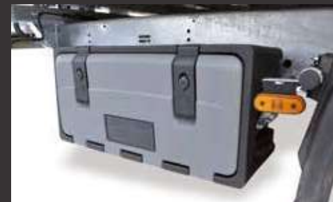
Plastic toolbox under the cargo bed
