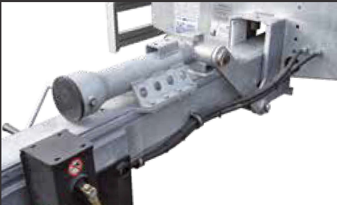
Horizontal height adjustment of drawbar
