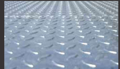
Steel chequerplate flooring
