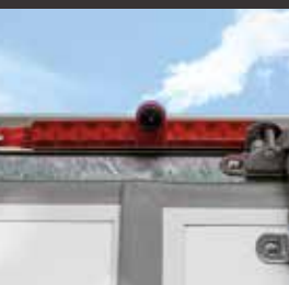
Third brake light with integrated reversing camera
