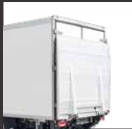
Liftgate in front of the tailgate (different manufacturers)
