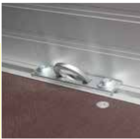
Lashing points in a groove
