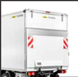
Liftgate with top tailgate (different manufacturers)
