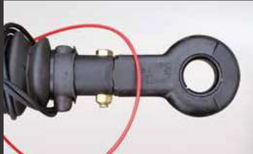
DIN tie-down eye for height-adjustable drawbar
