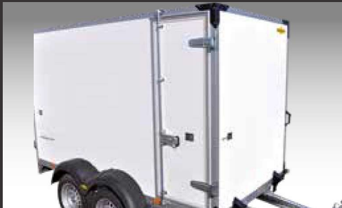
Side door with espagnolette lock, from internal height 1500–2300 mm
