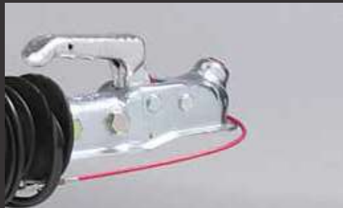
Ball head coupling for height-adjustable drawbar
