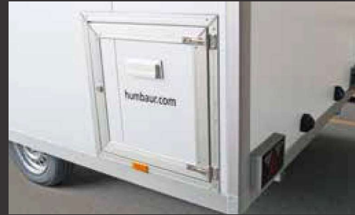
Gas cylinder compartment with outer door
